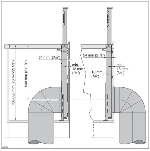
Exhaust air ducting to the front.
